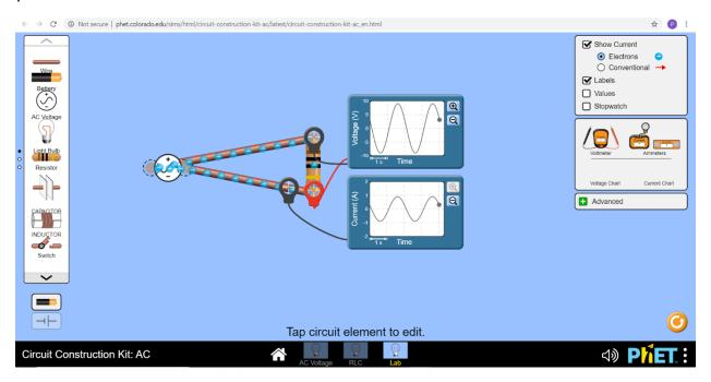
Notice that I have placed the voltage chart and current chart on top of each other. You can see that the voltage and current are rising and falling together, as you'd intuitively expect for a circuit with a power supply and a resistor. You can adjust the scale of the current and voltage
