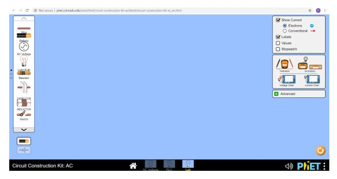
Now move an AC voltage source into the blue part of the screen by dragging it from the white component box on the left. Move a resistor out into the blue part as well, and then connect the AC source and resistor with two wires – also dragged from the white component box. When the connections are made, electrons (!) will appear in the circuit and they will wiggle back and forth.
