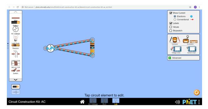
Next set up the "Voltage Chart" and "Current Chart" to read what is going on in the circuit and to see the dependence on time. To use the voltage chart, connect the two contacts across a component. To use the current chart, just place the contact at a point in the circuit. Arrange your screen as shown below:
