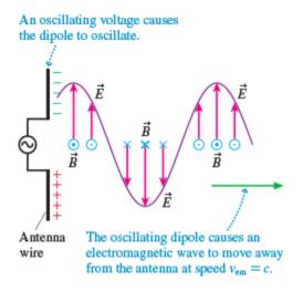
As the illustration from your textbook above shows, a radio antenna works by sloshing charge back and forth, giving an oscillating electric field and (because moving charges produce magnetic fields) an oscillating magnetic field.
