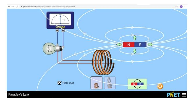
The voltage meter at the top of the screen will be your EMF measure, while the light bulb will tell you when there is current flowing through the circuit. You will see the magnetic field lines going through the coil near the center of the screen, and that will give you a qualitative measure of the magnetic flux.
