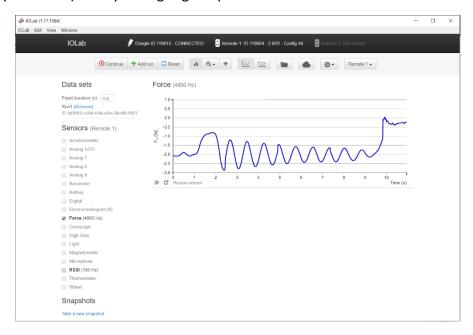
Determine the period of the oscillations by measuring the time over which a series of reasonable-looking oscillations take place.
