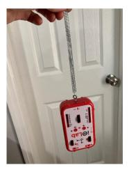
With the force display on in the iOLab app, start recording data and pull the iOLab down so it begins to oscillate. Let it oscillate until the amplitude of the oscillations has gotten considerably smaller, and then stop recording. If your hand-eye coordination is no better than mine (and that is a very low level) then you might get a plot that looks like this:
